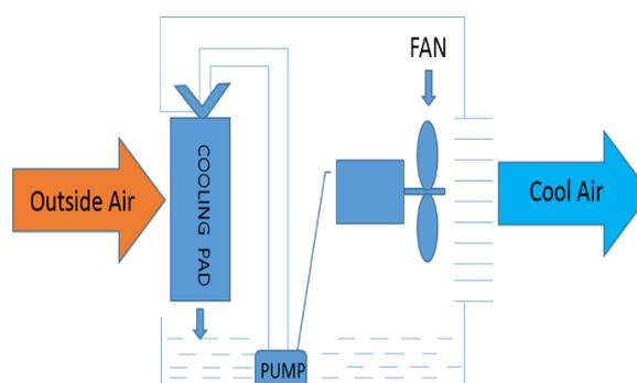
Fig.1.1: Schematic diagram of Desert cooler
