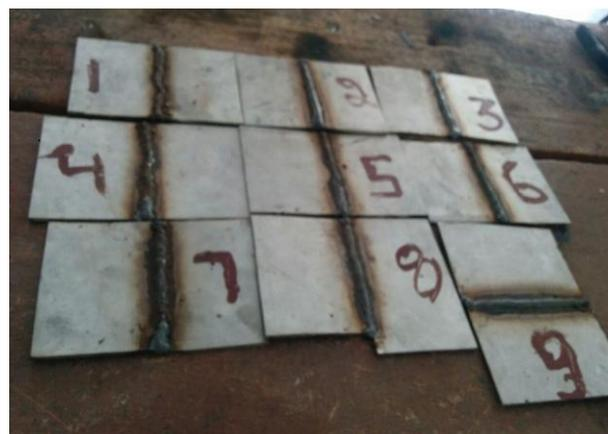
Figure4. Welded specimens for testing
