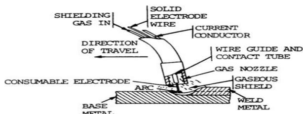
Figure2. MIG welding process<sup>[11]</sup>
