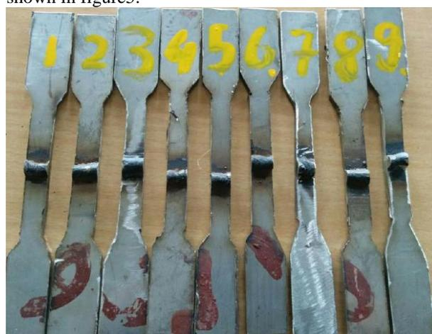
Figure5. Specimens for Testing in UTM
