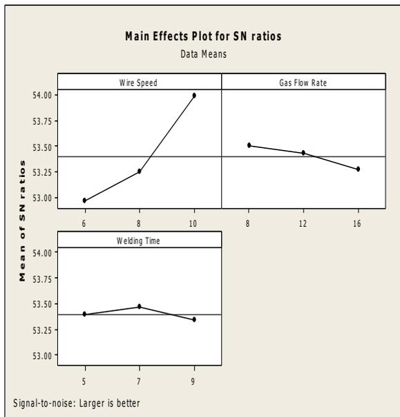
Figure6. Main Effect Plot Graph of S/N ratios of Hardness
