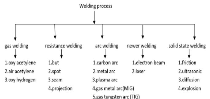
Figure1. Different types of welding techniques.
