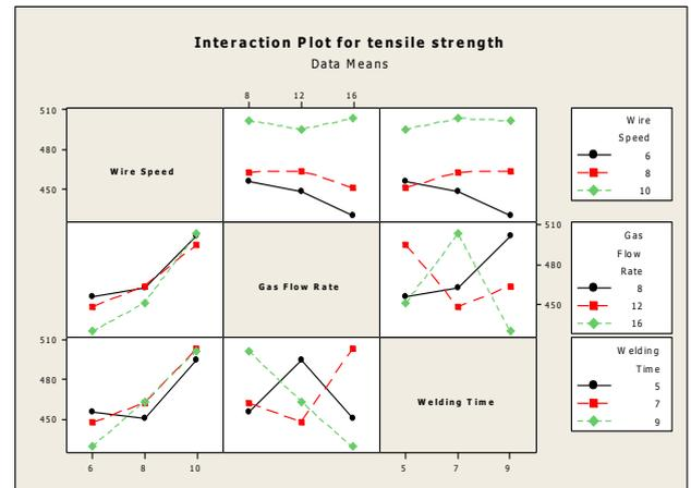
Figure7. Interaction plot between all the three input parameters and tensile strength
