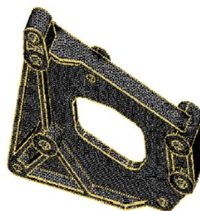
Fig 9: Tetrahedral meshing of the modified mounting bracket
