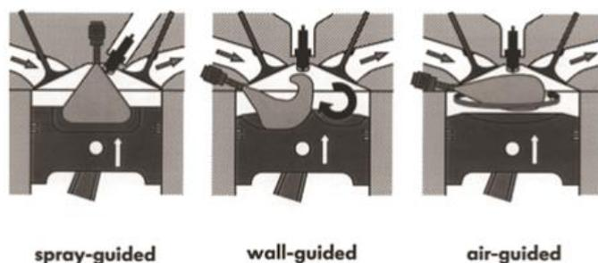
Fig. 1. Injector Spark plug arrangements
